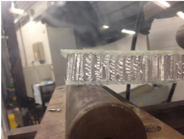
Figure 19: Failure of epoxy used to bond the glass fibre skins and honeycomb core together during GF-H-3-B2 bending test. Failure is shown through the sliding of the top facesheet.
