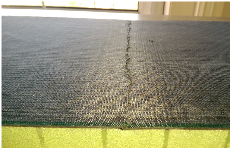
Figure 50: CF-F-5a-B facesheet failure. Note similarity to failure on CF-F-3-B panel.
