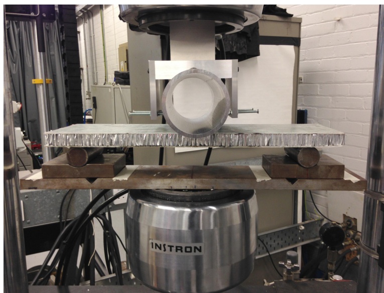
Figure 16: 3 point bending rig with GF-H-3-B panel.
