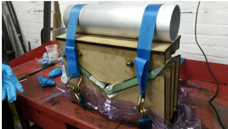
Figure 72: Cut-and-fold bending jig in closed configuration, used for creating joint panels with a 65 degree bend.
