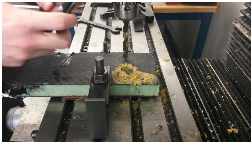
Figure 77: Holes being drilled into a joint panel to accommodate the metal sleeves.
