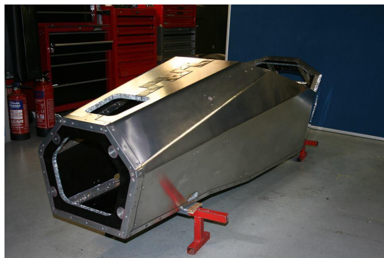
Figure 4: Example of a cut and fold monocoque chassis.
