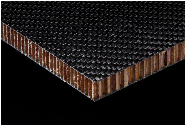
Figure 5: Sandwich panel with carbon fibre skins and Nomex core.
