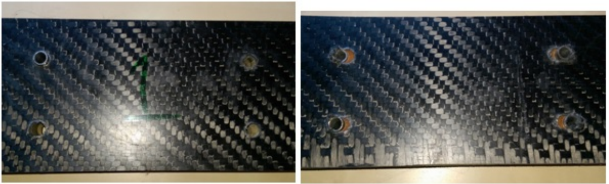
Figure 79: Movement of the inserts caused by continued tension of insert test, with CF-F-3-I1 (left) stopped after the first drop in load and CF-F-3-I2 (right) continued.
