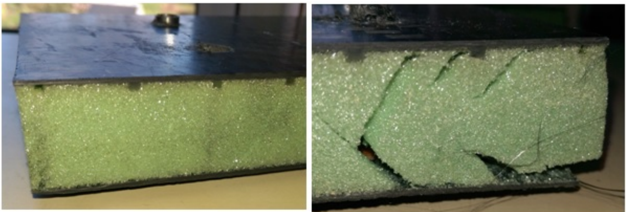
Figure 80: Damage caused by continuation of insert test, with CF-F-3-I1 (left) stopped after the first drop in load and CF-F-3-I2 (right) continued.
